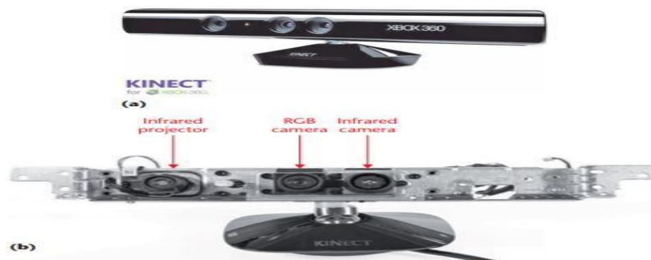
Figure 1. Microsoft Kinect sensor. (a) The Kinect sensor for Xbox 360. (b) The infrared (IR) projector, IR camera, and RGB camera inside a Kinect sensor.
